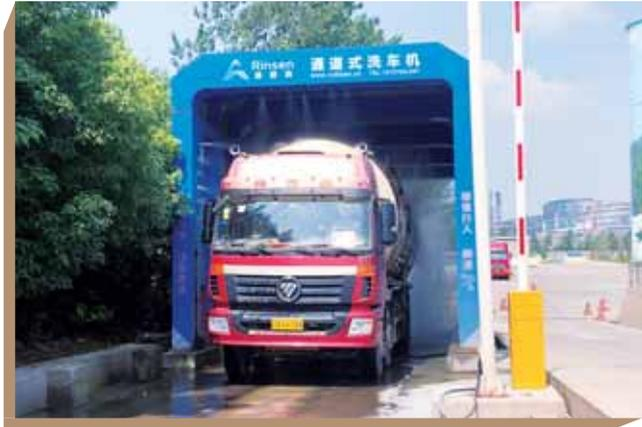
*Automated Truck Washing Machine at Nanjing Nangang Slag Plant*
